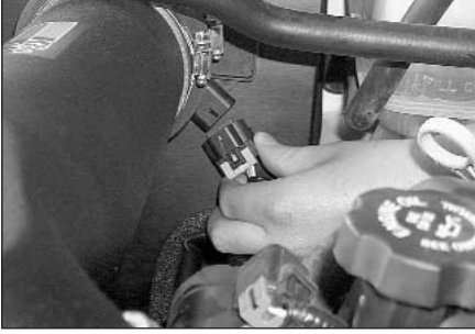
15. Re-connect the mass air sensor electrical connection as shown.
