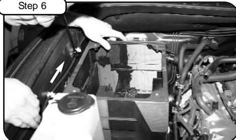
Install filter adaptor to new housing with button head screws provided. Install new housing using screws from step 5.
