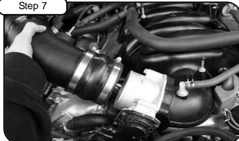
With couplers and clamps provided, place onto new intake tube and install. Make sure 4-1/4" coupler is on filter side and 3-1/2" coupler is on throttle body side.
