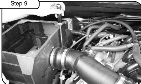
Tighten clamps with 5/16" nut driver. Take out OE crankcase line and replace with 1/2" hose and clamp provided.
