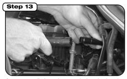
Connect supplied vent hose to nipple at intake tube and at breather vent tube.
