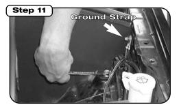
Use ground strap hardware for inner fender for mounting.
