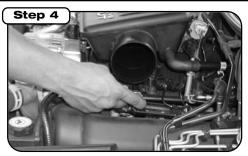
Unbolt resonator at manifold (Two bolts, opposite sides).
