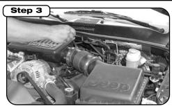
Loosen clamp at air resonator box and remove top half of filter box.
