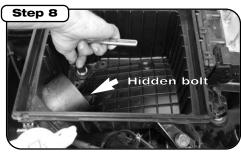
Remove four bolts from lower half of air box.
