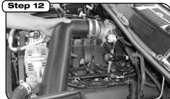
Thread filter end of housing through opening in filter housing first, then slip coupler over throttle body. Tighten clamps at throttle body.
