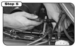
Remove vent hose at tubing coupler.
