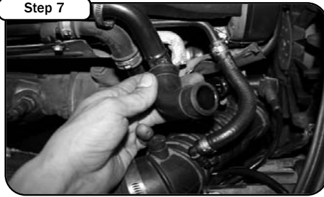
Step 7 Remove clamps holding second breather from top of factory tube. Save elbow for later use.
