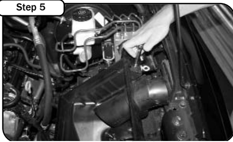
Step 5 Remove the 10mm bolt on the side of the air box set aside for later use. Lift the lower air box up and out of the engine bay.
