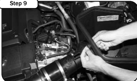
Step 9 Slide the intake tube assembly into the housing. Secure the tube to the housing with the supplied M6 hardware. Tighten and secure the hose clamp.
