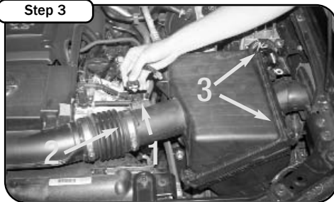
Step 3 Disconnect the MAF sensor (1). Loosen the hose clamp on the air box(2), and unclip the upper portion of the air box(3).
