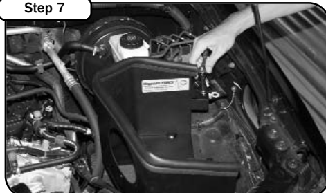
Step 7 Place the rubber trim seal along the edge of the housing. Lower the housing into the engine bay secure housing with the bolt removed in step 5.
