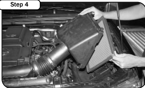
Step 4 Remove the upper portion of the air box and the factory air filter.
