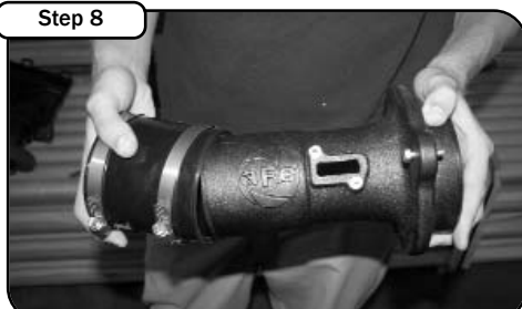
Step 8 Place the coupler on to the intake tube. Do not tighten clamps at this time.
