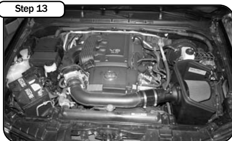
Step 13 Place enclosed CARB EO sticker on a clean/smooth surface on or near the intake system. EO identification label is required in passing the Smog Check inspection. Your installation is now complete. Make sure you tighten all clamps and check all electrical connections. Re check periodically
