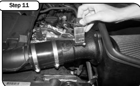
Step 11 Transfer the MAF sensor to the aFe intake tube. Secure with the supplied gaskets, spacers, and screws. Make sure you pay attention to the direction of the arrow on the MAF sensor.
