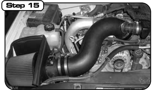
Step 15 Complete Stage 2 kit installed. Make sure all clamps are tight and all components are secure. Check and retighten connections and filter after a few hours of operation.
