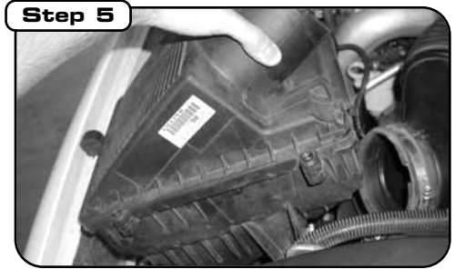
Step 5 Remove the complete stock air box from the rubber mounts. Pull up and slide sideways toward radiator.
