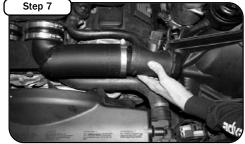
Install mass air sensors into the tube by pressing the sensor onto the tube. Tighten down provided #52 clamps.
