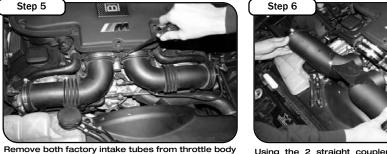
Using the 2 straight couplers provided in the kit install the high flow aFe intake tube.
