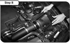
Install both air boxes using reducer couplers. Attach factory clips to secure to the air box and tighten clamps at coupler.
