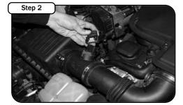
Unplug both Mass air sensor plugs from sensors.
