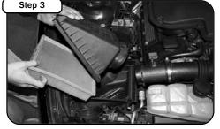
Remove clips from the mass air sensor and the air boxes and remove top half of air boxes and filters.
