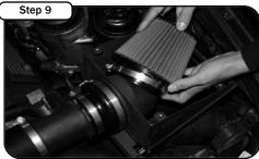
Install 2 provided High Flow aFe filters and tighten clamps.
