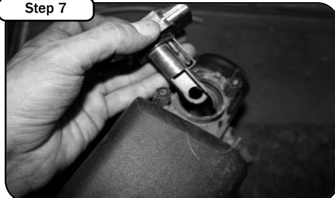
With phillips screwdriver, carefully remove the MAF sensor from OE air box.
