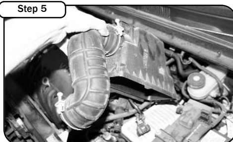
With 10mm socket or phillips screw driver, loosen OE intake tube. Pull crank case line away from intake tube. Remove upper half out of vehicle.
