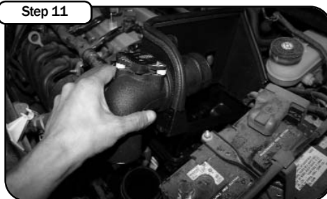
Install housing w/ tube into stock lower OE air box. Guide the housing tabs into the two OE air box slots. Place tube into coupling from step 10 and tighten using 1/4" nut driver.
