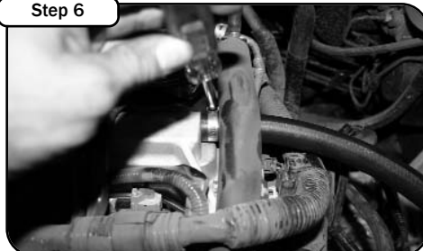
With 10mm socket, loosen the 4 nuts holding the engine cover and remove. Replace the crankcase line with the 5/8" hose provided and mini clamps. Tighten using 1/4" nut driver. Re-install engine cover.
