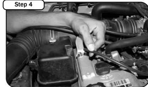
Disconnect and remove both vacuum lines from factory tube and loosen both clamps with 10mm socket or wrench.
