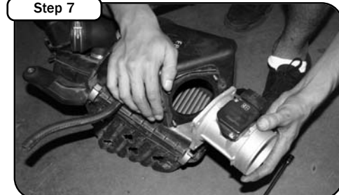
With 10mm socket or wrench carefully remove factory MAF sensor. Remove factory rubber gasket.
