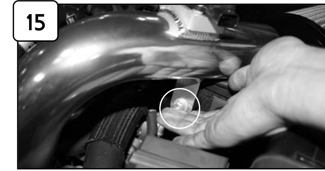
15 With M6 nut, wavy and flat washer provided, secure tab and tighten using 10mm socket or wrench.
