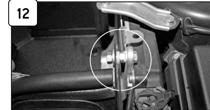
12 Attach tab on housing to screw on ECU bracket. Make sure nylon spacer is between tab and ECU. Secure tab using M6 nut, wavy and flat washer. Tighten using 10mm socket or wrench.
