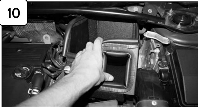
10 Install housing and position grommets on housing to factory fittings.
