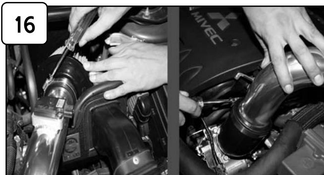
16 Install filter and tighten using 5/16" nut driver. Tighten all remaining clamps using 5/16" nut driver.
