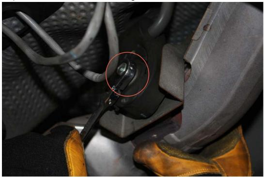
Step #4: Remove 12mm bolt on hanger.
