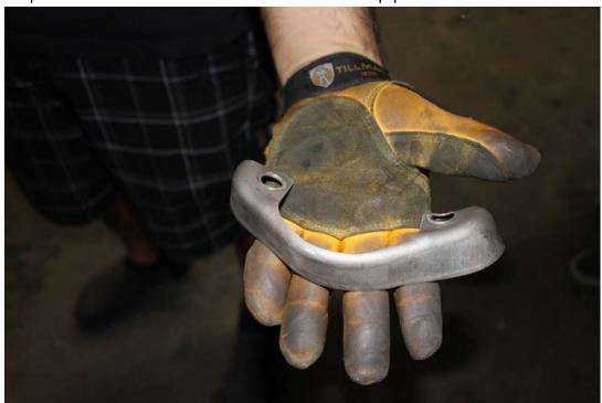
Step #6: Heatshield removed from OEM downpipe.
