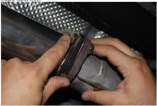
Step #12: Apply a very small amount of anit-seize on the O2 sensor threads. Screw O2 sensor into mechancial CEL fix and tighten.
