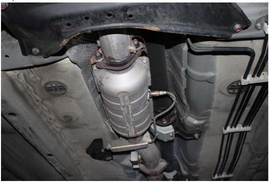
Step #2: Remove 19mm nuts on front of cat.
