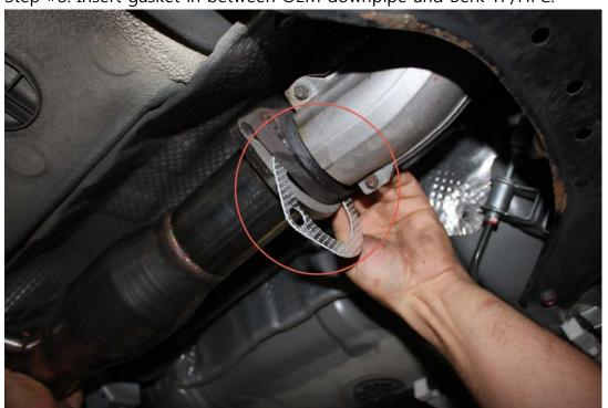
Step #8: Insert gasket in between OEM downpipe and Berk TP/HFC.
