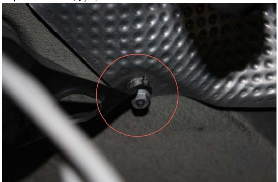
Step #13: Remove (Qty 2) 10mm nuts on O2 sensor wire cover.
