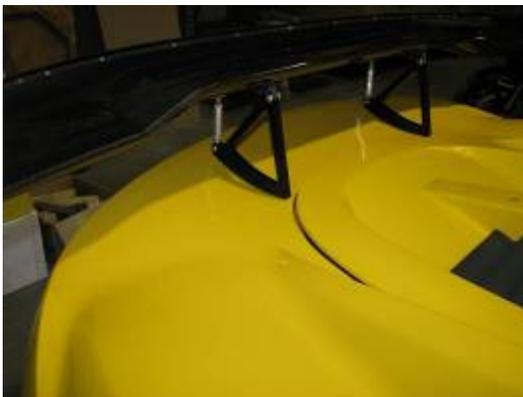
20. Re-attach the remaining wing components to the pedestals.
