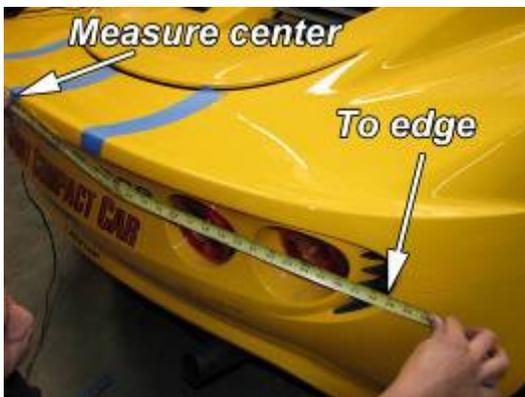
3. Use measuring tape to measure from the center line to where the edge as shown. It should be approximately 29". Make sure the distance is the same on both left and right sides. Then mark the true center on the center tape with a marker.
