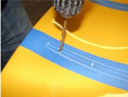
11. Now that the holes are marked, drill through these points using a 1/4" drill bit.
