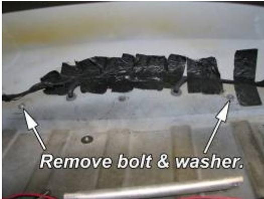
1. Remove factory bolts and washers from inside the trunk as shown.
