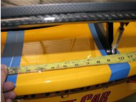
4. Assemble the upper brackets, pedestals, and adjustment rods to the wing. Tighten the bolts/nuts just enough so there is no play in the pedestals.
