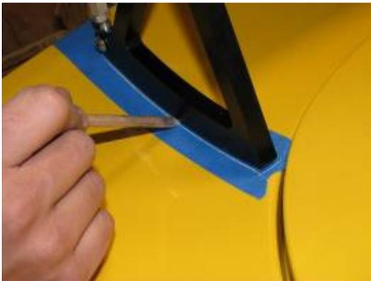
7. The front corner of the pedestal should be 0.5cm from the trunk lid gap.
