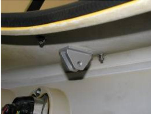
15. Secure each front and rear studs using a nut and a washer.
