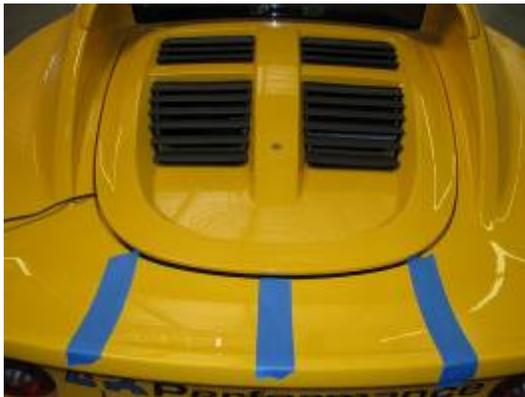
2. Apply masking tape to the center, left, and right as shown. The left and right tape placements are approximate (above the removed bolts and washers).
