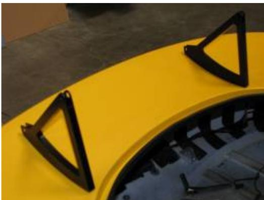
13. Insert the studs into the front and rear holes at the bottom of the pedestals. Make sure the hex keys on the studs are accessible.
