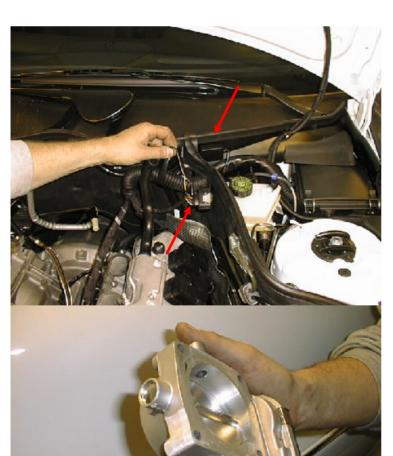
It is necessary to clamp the output voltage of the mass airflow meter.
