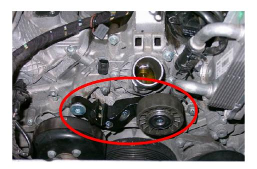
Fit the Kleemann support pulley wheel to the bracket and fit the belt
