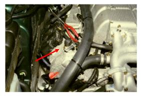
Remove the 4 rubber mounts from the valve covers.
