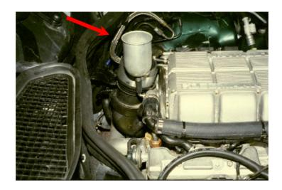
Fill the intercooler system with a 50/50 mix of antifreeze and water. It is important to always use a 50/50 mix even in warm climates as the antifreeze inhibits corrosion of aluminium parts. If the car is raised in the back the air will then move towards the reservoir hence the refill will be a lot quicker. This will also relieve the system of trapped air pockets.
