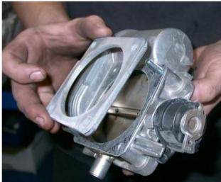
Remove the throttle body from the original manifold and install it onto the KLEEMANN manifold. Use the screws and the gasket supplied from the kit. The longest screw is placed where the arrow point on the next picture
