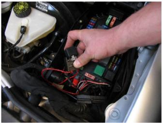
A wire is drawn form the pump+ to the relay box where it is joined in the kit relay as shown.
