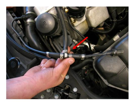
Cut the coolant line from the expansion tank. Install the plastic T-piece connection. Connect the supplied hose between the third leg of the connector and the outlet water manifold stub on the back of the SC. (One Way Valve has to be fitted also so do not connect to the stub yet.)
