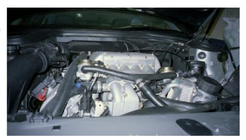
Grind the aluminum housing of the dash pots so they fit back onto the KLEEMANN intake manifold.
