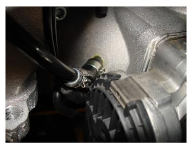
Connect the supplied hose to the 8mm pipe on the inlet housing using the supplied cobra clamps, in order to connect the tank ventilation. Next to the 8 mm tap there is two 4 mm taps. Mount the vacuum line so that it is long enough to reach the front of the compressor.
