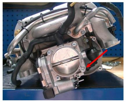
Remove the vacuum dashpot from the front of the original manifold. Exercise caution when removing the actuator arm. The mounting holes of the vacuum dashpot are not in the correct orientation so as to operate the bypass valve. You will have to modify the vacuum dashpot mounting in order for it to fit the KLEEMANN Compressor System:
