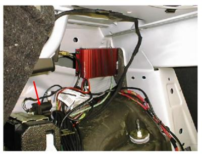
The C W203 has an in-tank centerfugal fuel pump. This pump is not able deliver enough pressure for proper fuel mixtures for full boost at high engine speeds. The pump booster gives the fuel pump 17VDC when boost pressure is present.
