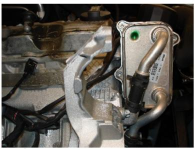
Cut the bracket down the middle as shown
