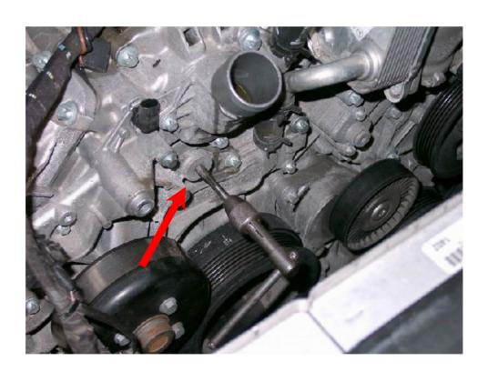
A M8 tread has to be made in the O.E. water pump to fit the Kleemann bracket, use the long M 8 torx bolt from the O.E. pulley wheel in the other side.
