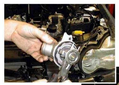
Remove the thermostat with a pair of needle nose pliers. It is important to remove the thermostat as shown in the picture or permanent damage to the thermostat will be the result!
