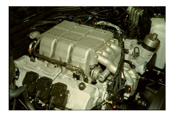
Install the EGR valve (you may need to grind a small portion of the EGR valve body for clearance). Install the EGR pipe.
