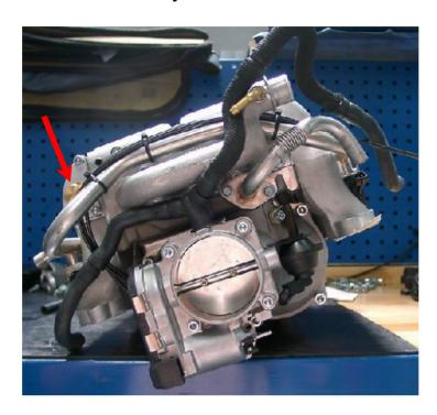
Carefully heat the end of the plastic vacuum hose that runs from the Brake booster to the engine and pull out the white snap on connector that is fitted on the original hose. Heat up the plastic vacuum hose again and push the supplied vacuum connector on to the vacuum line while it is hot, so it is a tight fit.
