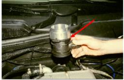
Install the original 90 degree intake hose on the throttle body.
