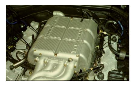
Re-route the engine wiring harness so that it passes under the water manifold. Reconnect all plugs to their original locations. Use zip ties to secure the engine wiring harness to the fuel rail.
