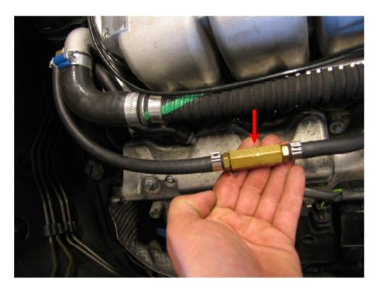
Mount the One Way Valve between the hose coming from the third leg of the T-piece and the SC. Important; the arrows on the valve ( red arrow ) MUST be pointing towards the SC outlet. (One Way Valve must be assembled using Thread sealing )
