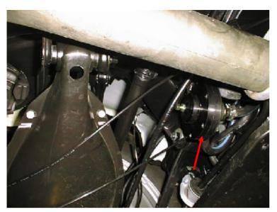
Install the KLEEMANN fuel regulator using the bracket.
