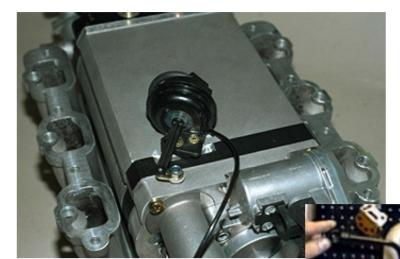
From this point forward, is important to never rest the weight of the compressor on the vacuum dashpot.
