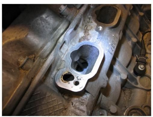
make sure that nothing have entered the ducts, like some of the screws from the O.E. manifold
