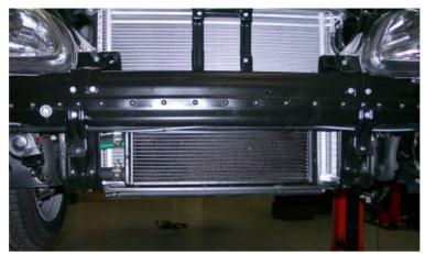
Remove the front bumper. You may have to remove some of the radiator covers for access to install the KLEEMANN radiator. Install the KLEEMANN radiator as shown in the picture. On some models the O.E radiator has to be lifted in order to install the intercooler. On other models the intercooler can be bolted directly on to the front bridge.
