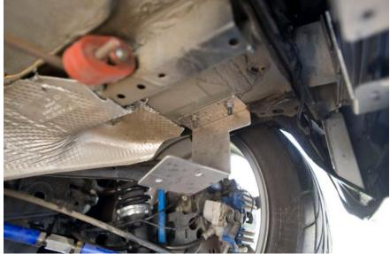
The two large front brackets attach to these posts as shown in the image above. A step drill may be required to open up the mounting points. Install the brackets and tighten down the nuts to 25 ft-lbs each.
