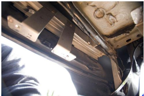
When the correct location has been determined, use a marker to trace the outline of the brackets on the tunnels. Mark out where the brackets sit on the bumper. Mark the bumper level on the brackets. You should be able to drill at any point above this line. Looking at the bumper from the side, however, shows that some parts of the bumper are thicker than others (keep that in mind when deciding where to drill).
