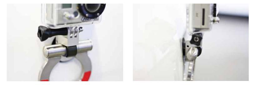
To install, Simply remove the tow loop from your Rennline Tow hook. Slide the GoPro mount onto the screw as shown in Photo 1 and tighten the supplied set screws using the supplied hex key. Next, reinstall the tow loop using the instructions included in the tow hook kit. Lastly mount the GoPro to the Rennline GoPro mount making sure to tighten the GoPro thumb screw tight enough.
