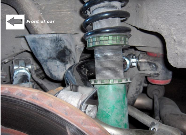
The rear upper arms should be installed with the tubing closer to the traction rod, towards the front of the car, as shown
