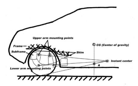
The following diagram shows what happens when you raise the subframe closer to the chassis. For this example, we are comparing what happens to the anti-squat when the ride height remains the same. When the subframe is raised, the rear "instant center" is raised as well, that moves point A up and increases anti-squat.
