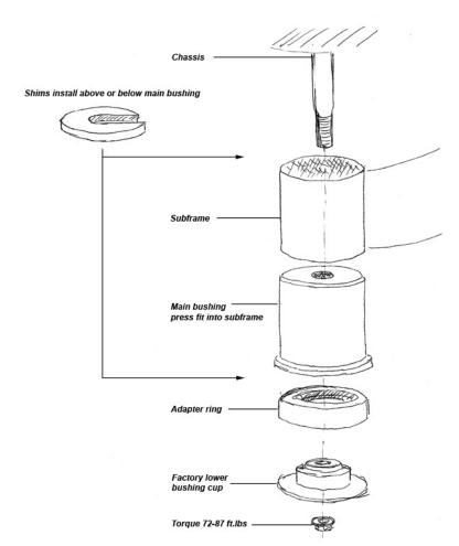
Remove subframe and OEM subframe bushings. The OEM subframe bushings can either be pressed out or cut out. The entire OEM bushing must be removed, including all the outer metal "shells" (race). When the OEM bushing is completely removed, there should just be 1 ring of steel left that is part of the subframe itself.
