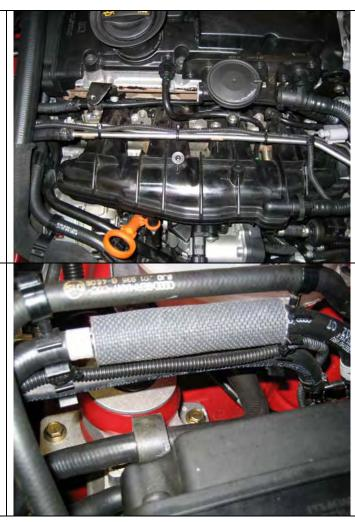
Connect the extension harness to the OEM connector for the Turbocharger Recirculation Valve N249 (near the turbocharger). Zip tie the connector to the A/C pipe on the passenger side of the vehicle, forward of the ABS pump. Place the connector over the rubber buffer on the A/C pipe before you zip tie. Use two zip ties, one at each end of the connector.
