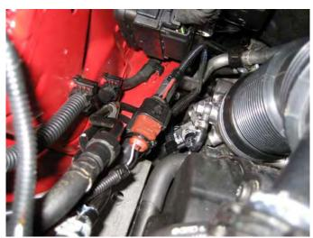
Install supplied hose for the Turbocharger Recirculation from the Recirculation Valve flange, under the A/C service hose, to the Turbocharger Inlet hose. Attach support clip to coolant service line above alternator. Install spring clamps at both ends of the hose.
