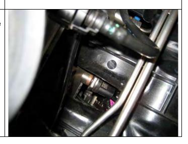
Disconnect electrical connector for Camshaft Position Sensor G40. There is a small plastic support clip attached to the fuel rail on the wiring loom as it leads under the intake manifold. Detach this from the fuel rail.
