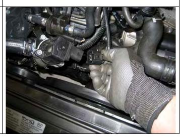
104 Run the extension harness along the EVAP and Fuel hard pipe on the intake manifold.
