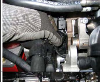
Using a small ¼" drive T-30 Torx socket, remove the 5 upper bolts fastening the intake manifold to the cylinder head. Two additional lower bolts are accessible just above and to the left and right of the Throttle Control Module. An additional two M6 nuts are located on the underside of the cylinder 1 and 4 intake runners.
