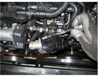
103 Connect the supplied electrical harness extension to the Turbocharger Recirculation Valve N249.
