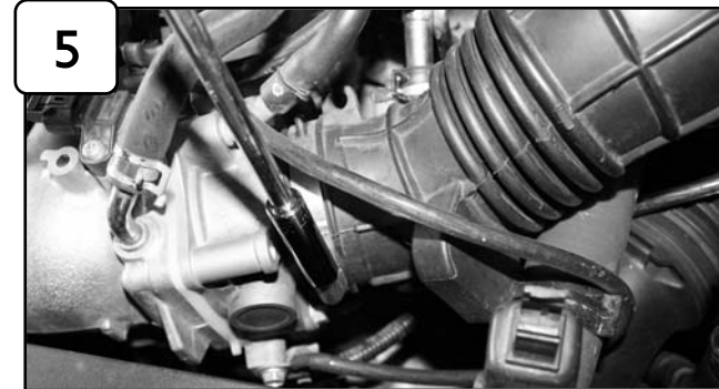
Loosen the clamps on stock intake tube using 10mm socket. Pull back vacuum line and crank case from intake tube.
