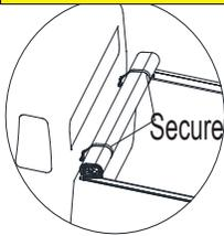
Before driving with cover open, **BOTH STRAPS MUST BE SECURED TO RETAINER LOOPS.** Failure to do so could cause accidental release of the cover, resulting in personal injury or property damage.
