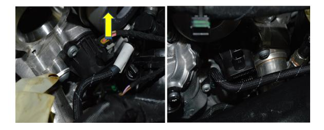
9. Ensure the supplied O-rings are in place on the base of the Forge Motorsport valves then attach the valves into the mounting position taking note that the valves are handed for the left and right hand turbo, this is to avoid interference with the turbos actuators. Use the removed torx fasteners on each valve to secure them into position.
