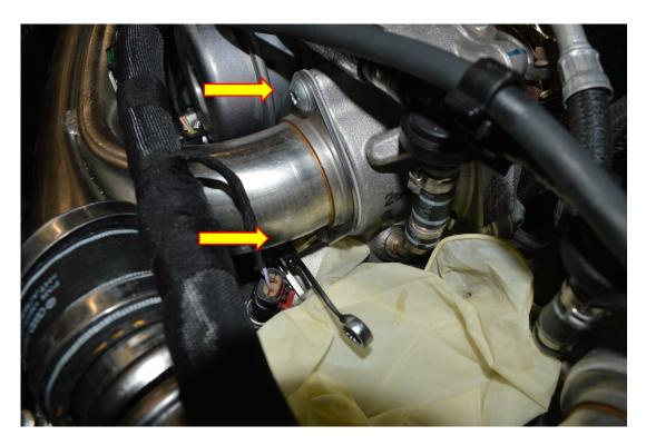
6. On the underside of the intake pipe there is a breather fitting that needs to be removed from situ, depress both the sides of the fitting while pulling the fitting away from the inlet pipe.
