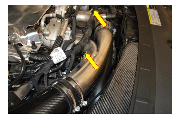
3. Using a 7mm socket or flat bladed screwdriver loosen the hose clamps arrowed below and slide the silicone joiner to the left as pictured below.
