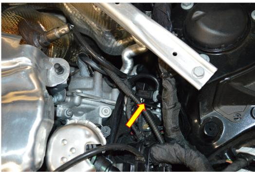
12. Next locate the vacuum source, which is situated below the throttle body on the right-hand side of the engine. There is a rubber hose cover which needs to be removed, this just pulls off. Once removed you will now be able to attach the remaining silicone hose to the vacuum hose and run it up to the solenoid. Use the small cable ties provided to secure all the silicone hose ends and prevent them from coming loose.
