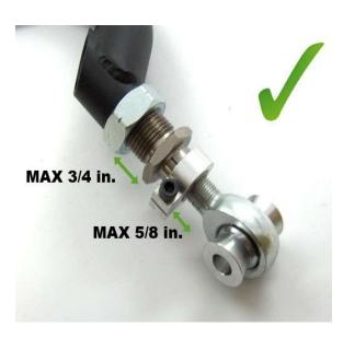
The next picture shows a properly threaded adjuster. The rod end (heim joint) will thread out about 2/3 the length of the adjuster. The maximum adjustment limits are shown in the picture.
