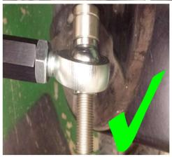
Note that the FK Rod End can rotate freely, so the picture on left is not binding even though the edge of the ball is touching the housing.
