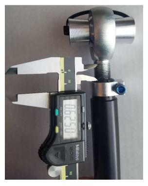
Once the FK Rod End is long/short enough, tighten down the Aluminum Clamps. Note that for safe thread engagement, the **maximum** amount of exposed thread on the Rod End should not exceed the measurement as pictured on the left.
