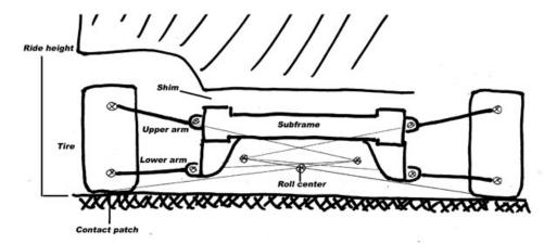
The following diagram shows the subframe raised closer towards the chassis (no more gap between subframe and chassis), and the ride height lowered the same amount. The roll center position is un-changed.
