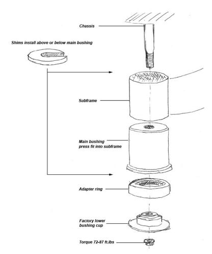
Remove subframe and OEM subframe bushings. The OEM subframe bushings can either be pressed out or cut out. The entire OEM bushing must be removed, including all the outer metal "shells" (race). When the OEM bushing is completely removed, there should just be 1 ring of steel left that is part of the subframe itself.
