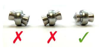
The advantage of the hybrid adjuster is that you can easily keep the rod end bearing centered during and after alignment. Make sure to keep the bearing centered as shown.
