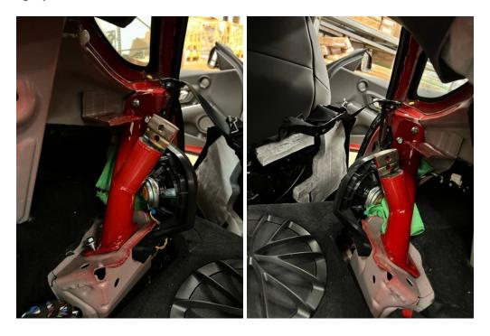
Now slide your new CMS roll bar in from the back hatch. Be sure to have a helper for this part as you don't want to hurt your back or damage your Supra. Line up the interlocking joints of the kick base plates installed in the previous step and install the bolts and nuts (but be sure to leave them loose)
