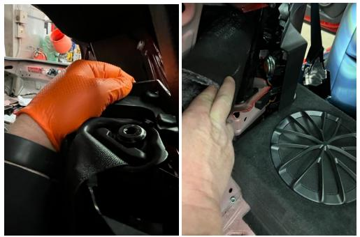
Remove the aluminum crossbar (one T50 torx bolt on each side) and also remove the support brackets (black aluminum rectangle tubes that run from the backside of the upper seatbelt mount down to chassis). A T12 torx bit will be needed.
