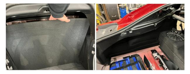
Now remove the rear trunk panel (two T30 torx screws as well as two push pins)
