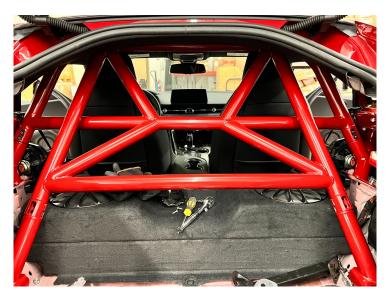
Time to start fine-tuning the interior trim. Mark out the  $\frac{3}{8}$ " holes that need to be drilled on the large side panel pieces for kicker placement.
