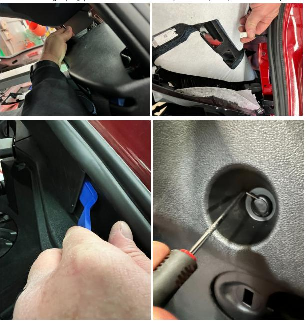
Followed by removing the trim from around top of seatbelt (just pulls out). Next pull the trim from the bottom of the b-pillar. ( two T20 torx screws on top then pull out ) you will have enough slack in the seatbelt to pull this out of your car to mark and trim
