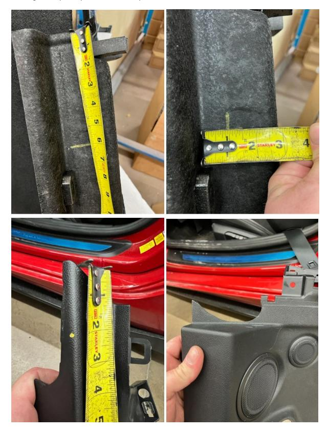
Remove the kicker plates to reinstall the trim and place the large side pieces back in their location (then re-install your kicker plates leaving the bolts loose). Tighten all interlocking bolts to 30ft/lbs, then tighten all 10 of the mounting bolts to 50ft/lbs.
