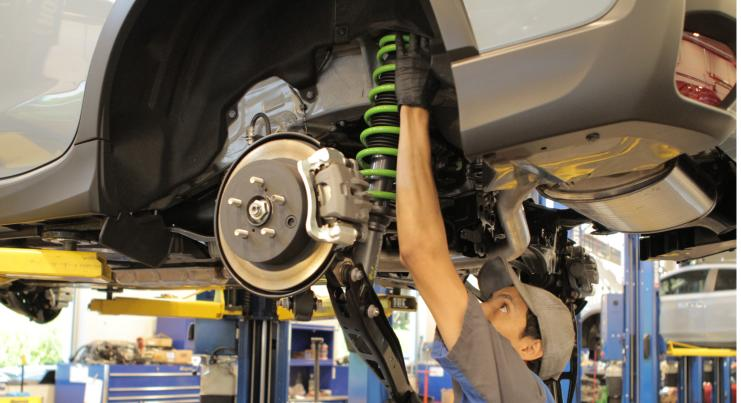
**SAFETY WARNING:** Installing suspension often requires special tools and expert knowledge. All fitment should be performed by a qualified and experience fitter. Always tighten bushed components after the vehicle is let down onto the ground at normal ride height, otherwise damage from torsional stresses can occur.
