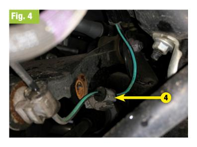
**5.** Remove the left and right gas tank protection shields and the handbrake cable retaining clips from the sub-frame front plates.
