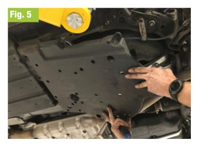
6. Support the rear sub-frame assembly with a Transmission jack or similar. (ensure you have clearance from the exhaust system).
