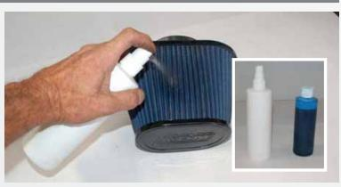
Wipe large debris from filter. Using the taller white bottle of cleaner from the kit, liberally spray the cleaner until it completely saturates the pleated material.
