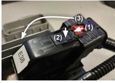
**STEP 5** - Take the E90 Unlock Cable. Attach both of its gray and blue ECM Connectors (A) to the top and bottom connector sockets on the ECM. Close their locking levers (3) until they click. The middle connector socket (black) will be left empty.
