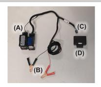
For your vehicle to accept tuning, you must perform a one-time unlock process on the Engine Control Module. With this Unlock Cable kit, you are able to unlock your own ECM using your tuning device without having to remove the ECM from the vehicle or ship it to us. Once the unlock is completed, you do not need to use the cable to install tunes or modify options, and will not need the unlock cable anymore.
