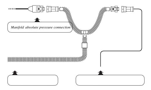
Disconnect the plug from the manifold absolute pressure sensor.
