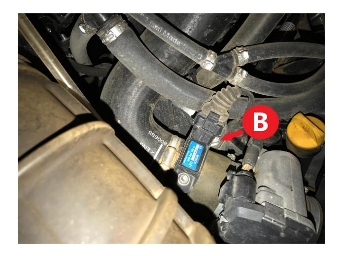
To begin, locate the turbo boost pressure sensor in your engine bay.
