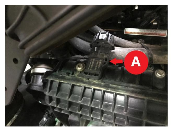
To begin, locate the connection to the manifold absolute pressure sensor in your engine bay.
