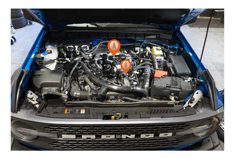
(A) manifold absolute pressure sensor(B) turbo boost pressure sensor
