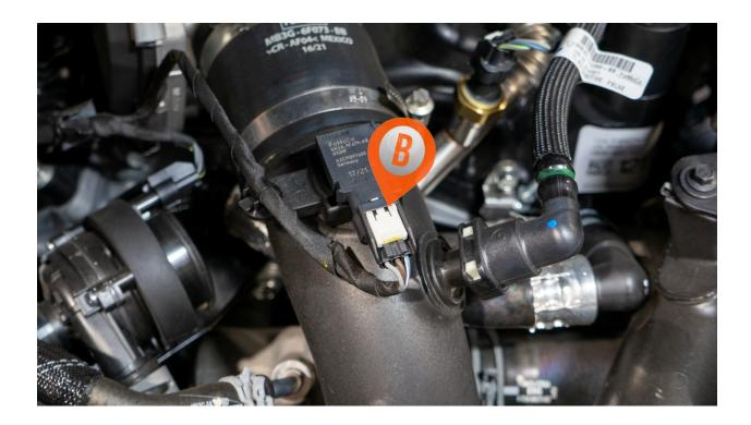
To begin, locate the turbo boost pressure sensor in your engine bay.
