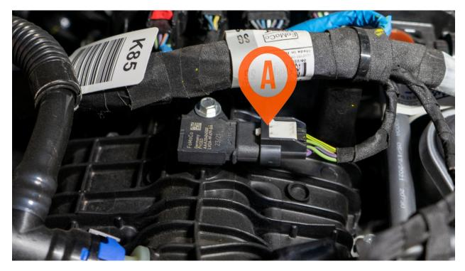
To begin, locate the connection to the manifold absolute pressure sensor in your engine bay.
