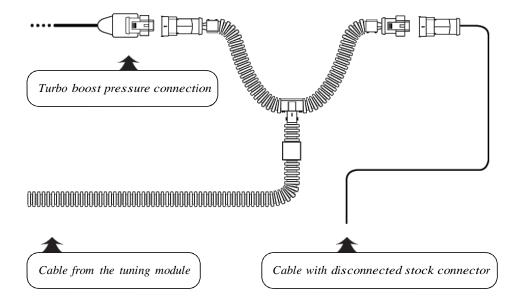
Disconnect the plug from turbo boost pressure sensor.
