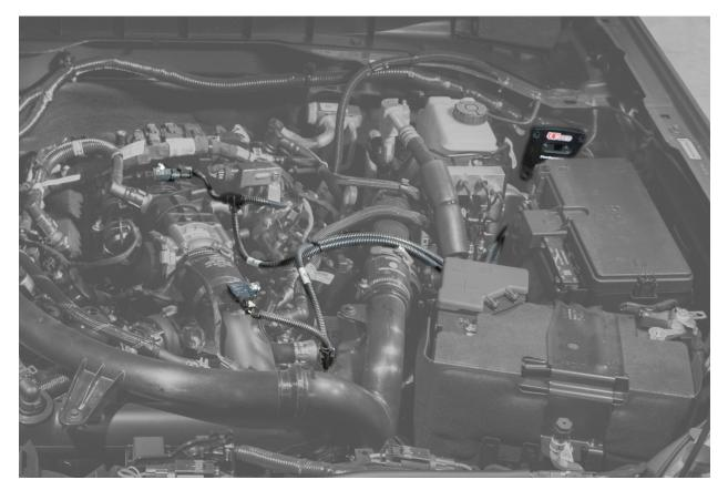
Step 4 - Connection to manifold absolute pressure sensor
