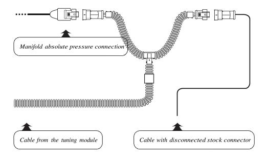
Disconnect the plug from the manifold absolute pressure sensor.
