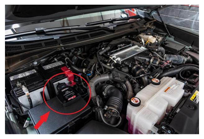
Step 8 - Fixing the tuning module and wiring harness
