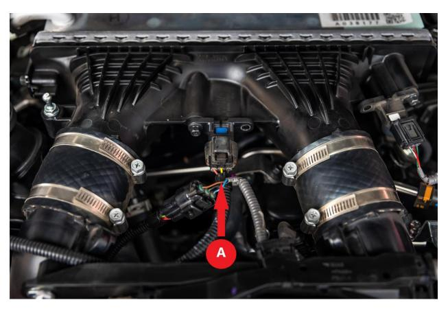
To begin, locate the connection to the manifold absolute pressure sensor in your engine bay.
