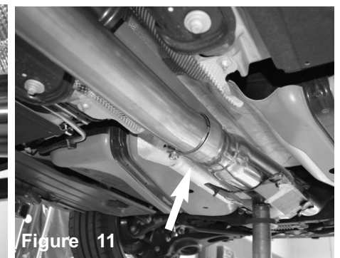
Figure 11 Secure the front pipe and mid pipe using band clamp, snug fit using 17mm socket and or wrench. DO NOT TIGHTEN!
