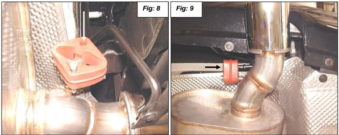
Adjust the muffler for best fit centering the exhaust tip in the bumper cut out. The rubber hangers should be angled forward as shown in figure 10. When the exhaust gets hot it grows in length and the hangers will hang straight.
