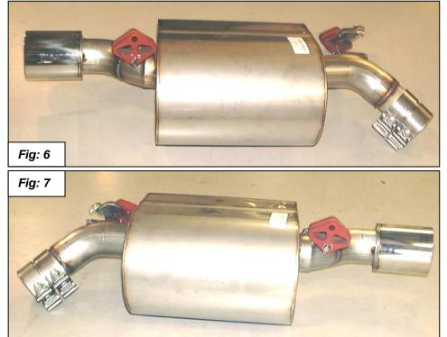
9. Install each muffler by sliding the clamps over the ends of the pipes. Attach the hangers to the car with the stock bolt and nut in the front and push the hanger over the stock rod in the rear as shown in figures 8 and 9.
