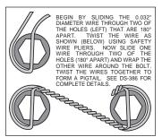
Figure 3. Safety Wire Diagram
