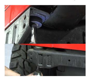
Again, using the 5/8" socket, remove the bolts that secure the body mounts in front of the gas tank.
