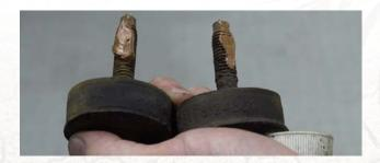
Reinstall all body mount bolts and torque to factory recommended specifications.
