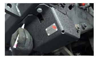
Using the 7/16" drill bit, drill a clearance hole in your bumper. Using a size R drill bit (.339" or similar), drill the starting hole for your self-threading bolt in your crossmember.
