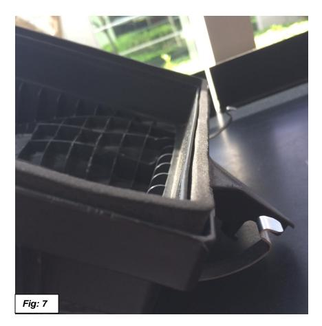
9. Remove the 4 clips from the lower airbox and install the 4 smaller clips supplied in the hardware kit. See Figure 8.
