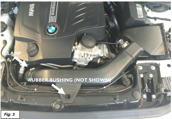
5. Remove lower airbox by gently lifting up. Remove filter. See Figure 4.
