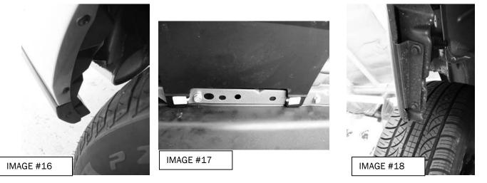
STEP 4) Lay the factory rear bumper on a clean surface. Locate and remove the factory clips and screws that secure the upper and lower half of the factory rear lower. Do not discard any of this hardware. It will be used in the installation of the new 3dCarbon rear lower.
