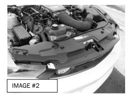
STEP 2) Carefully pull the bumper forward enough to access the wiring connectors on the side fog and marker lights. Disconnect the plug from the side marker lights. Locate and remove the air temperature sensor and relocate it as shown in images #3-5. Now remove the bumper completely from the car. Remove the front marker lights and the front grille from the bumper.
