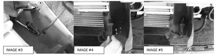
STEP 3) Remove the factory grille from the factory bumper. DO NOT DISCARD. It will be re-installed on the 3dCarbon front bumper. (See Images #6-8.)
