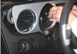
2. Locate the four locking tabs which retain the inner vent assembly to the cluster bezel. Carefully depress all four tabs to release the inner vent assembly.
