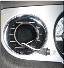
10. Make all necessary connections to the gauge and install the gauge into the VentPod until fully seated.
