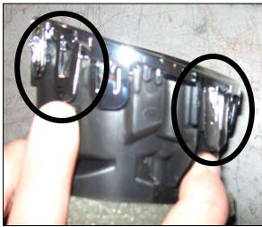
4. Once the trim ring has been removed, you must now remove both the primary and secondary air flow manipulators from the inner vent housing. Carefully pull up on each of the blades to release the posts from retainer pockets located on either side of the barrel. This step must be repeated for both the primary and secondary blade sets.
