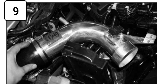
9 Install intake tube into vehicle and position tab to isolation mount and coupler.
