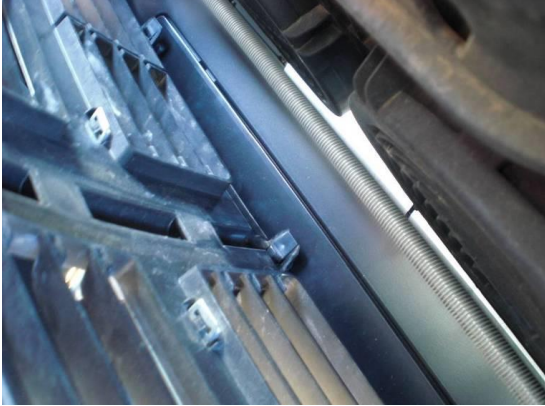
Figure 25: Stock grill installed on Aluminess door tabs
