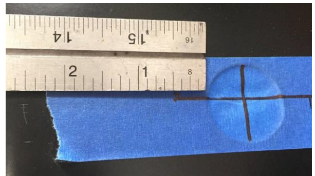
Figure 9. Measuring 0.5" out from each edge of sensor opening.
