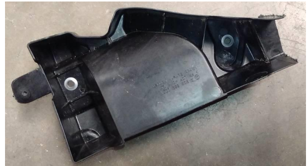
Figure 13. Plastic trim cut in half
