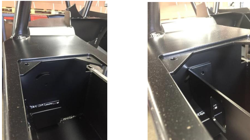
Figure 23. Install the crash sensor bracket in the orientation as shown.
