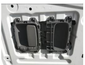
Figure 4. Torx bolts holding door handle on passenger side door.
