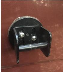
Figure 3. Latch pin assembly mounted on rear door.
