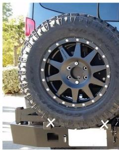
Figure 6. Rest tire on both support arms (before tightening the lugs or U-bolts down).
