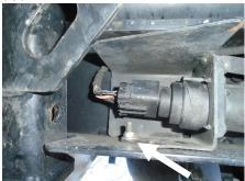
Figure 5. Tow Plug with ¼" button head screw.
