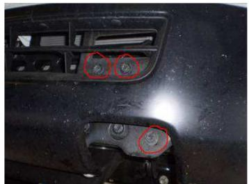
Figure 5. View from the from of the vehicle, 4 more bolts on the main bumper structure.
