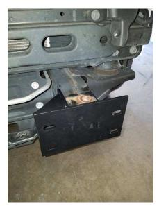
**Figure 9a.** Passenger side steel mounting bracket bolted onto frame. Note the orientation of the passenger vs driver side.
