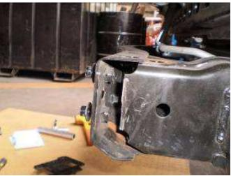
Figure 8a. Crossmember weld before cutting. Figure 8b. Crossmember weld after cutting.
