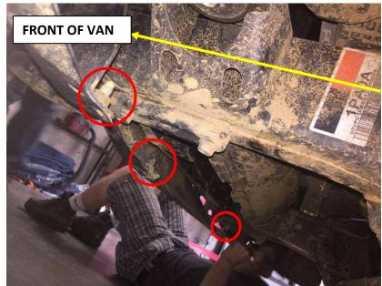
**Figure 4.** Bolts fastening the bumper to another support piece (4<sup>th</sup> bolt not pictured, out of frame to the left of the image)
