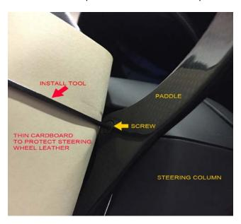
**Step 3:** In the reverse of Step 2, install the Carbonio carbon fiber paddle in the place of the original paddle. Again one screw will be easy to get to while the other will have very tight access. The following order works well:
