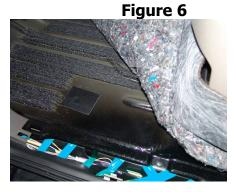
**16.** Secure F150 template over opening in front of driver's seat.
