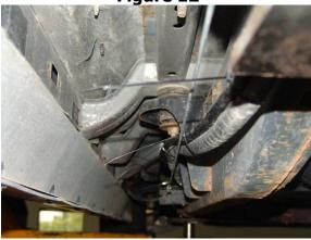
**22.** Loop any excess from the harness as shown and secure with zip-ties.
