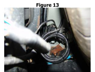
**23.** Line up the arrows on the top of the connectors, and plug the 4-pin camera harness connector installed earlier under the pickup bed into the 4-pin chassis harness connector.
