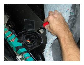
**19.** Recommended: Use a cotton swab or small brush to apply corrosion inhibitor to exposed edges.
