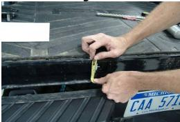
3. Center punch the mark and drill a pilot hole. Next, cut a 1-inch opening with a hole saw (Figure 3).
