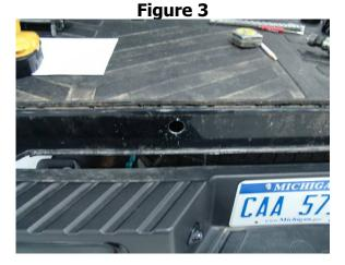
**4.** Clean the rough edges of the opening with a deburring tool. Recommended: Use a cotton swab or small brush to apply corrosion inhibitor to exposed edges (Figure 4). Reinstall tailgate.
