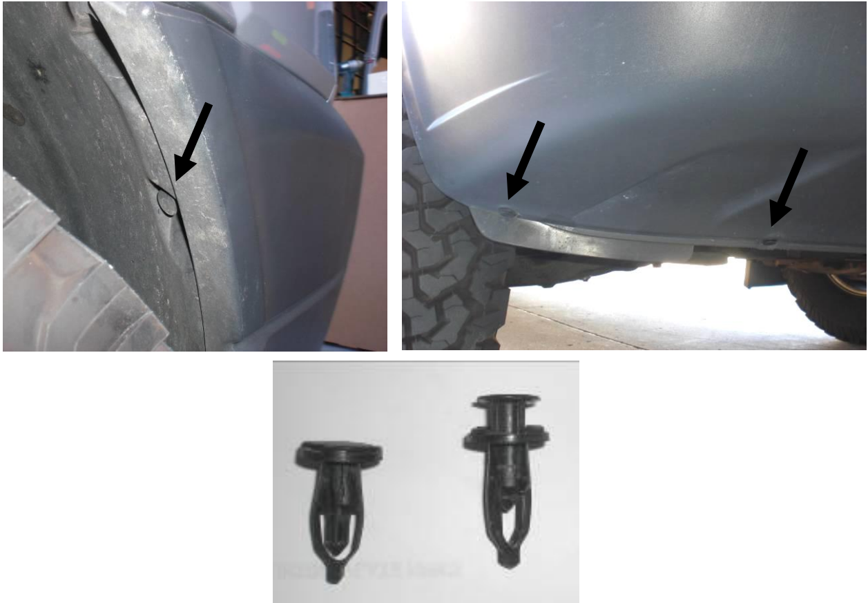
Figure 3. (Clockwise from top left) Plastic fastener location in fender well; Plastic fastener locations under leading edge of bumper; Plastic fastener closed (left) and open (right)
