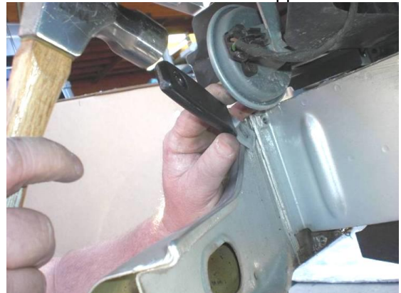
Figure 8. Releasing stock bumper with hammer and putty knife
