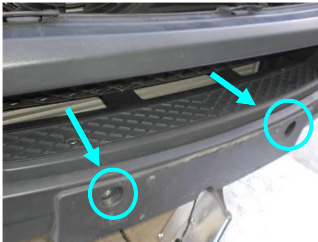
Figure 6. Plate cover (top) and plate cover removed (bottom) showing bumper cover fasteners
