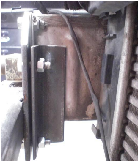
Figure 13. Attach the 2" X 1" angle brackets to the receiver mounting plates (this is the passenger side)
