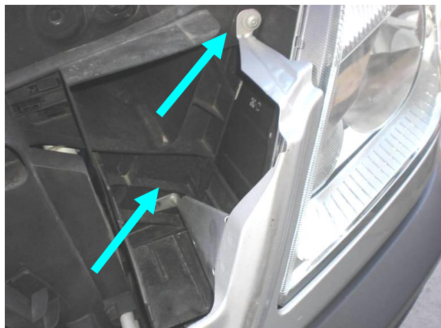
Figure 4. Headlight trim piece torx bolts
