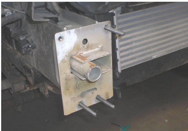
Figure 10. Frame profile after cutting.
