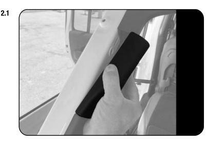
C Looking at the rear roll cage, remove the plastic trim covers located on the inside of the roll bar as shown.
