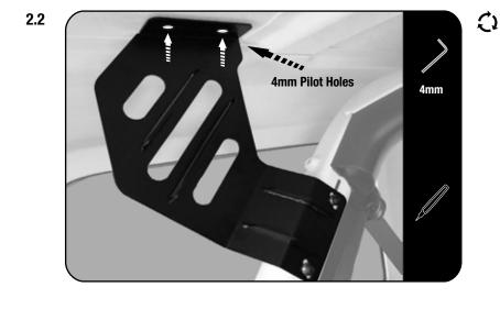
Fit the Inner Support Brackets (Items 6LH & 6RH) using the factory inserts in the roll bar, using M8 x 25 Button Head Bolts, M8 SS Spring Washer and M8 x 16 x 1.6SS Flat Washer (Items 16, 17 & 18). Refer to Figure 1.1 on page 3.
