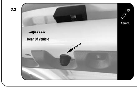
Open the rear passenger doors and locate the hole shown.
