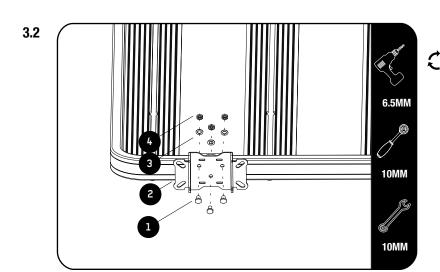
Drill a 6.5mm hole on the marked positions.
