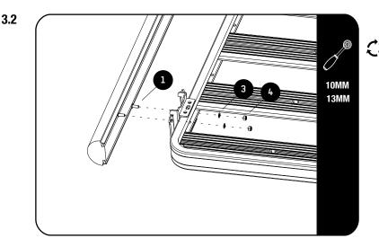
Depending on the type of Awning Extrusion, slide either three M6 x 16 Hex Bolt or three M8 x 20 Hex Bolts (Items 1 or 6) into the top slot and three into the bottom slot of the extrusion.
