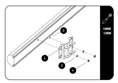
Depending on the type of Awning Extrusion, slide either three M6 x 16 Hex Bolt or three M8 x 20 Hex Bolts (Items 2 or 6) into the top extrusion slot and three into the bottom extrusion slot.
