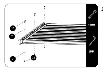
Position the Awning onto the Slimline II Rack with the help of a friend. Secure the center Mounting Bracket first.
