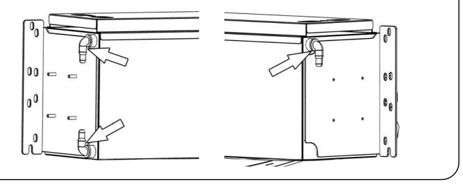
(**B**) Clip the Pump Elbow and Pump Filter (Items 7 & 9) into the Pump (Item 8) as shown.
