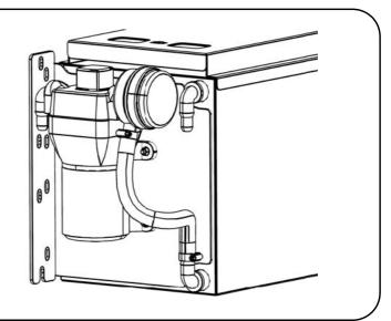
$\left( \ {\bf E} \ \right)$  Loosen and remove the eight bolts at the rear of the Drawer System as indicated by the arrows.
